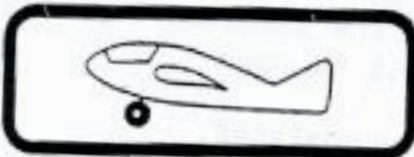
Landing gear retracted (lever aft)
