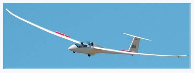
The Duo Discus was conceived as an advanced trainer with good cross country ability. It has a four piece unflapped wing with a modified Discus planform. The fuselage is derived from that of the two-place Janus. Approach control is by top surface airbrakes.
